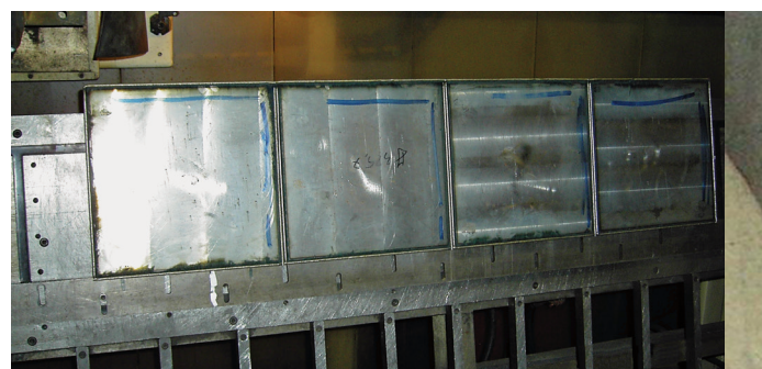
Ceramic moulds for tiles production Hardfaced with STELLOY 6-G
