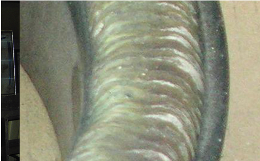
HP Valves - Ring Hardfaced with STELLOY 6-G
