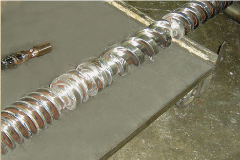
Extrusion screw Hardfaced with STELLOY 12-G
