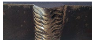
CAVITALLOY Welding position PE/4G
