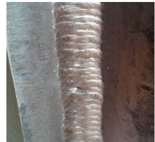
CHROMECORE 13 4-G Welding position PF/3F up
